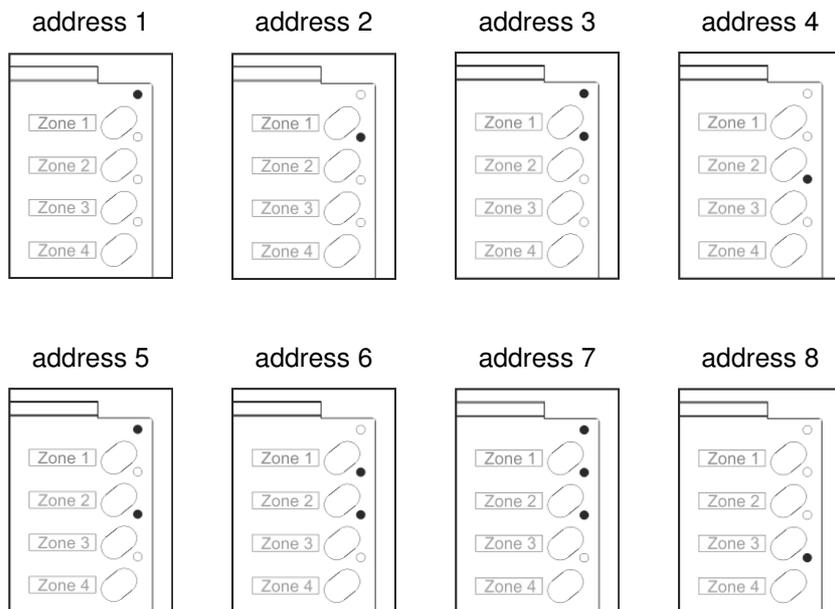
By pressing the “Zone 6” (5) key you can step trough the different address numbers.
